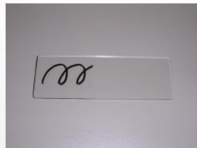
Ink of coating can be completely removed by wiping with tissue paper several times.
